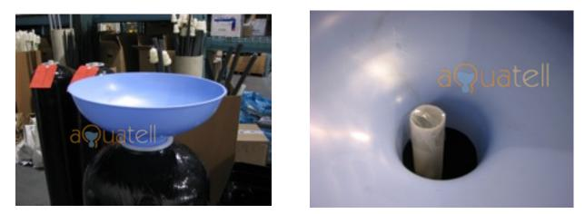
Once all of the resin has been added it is <u>very important to remove the piece of tape</u> from the top of the riser tube.
