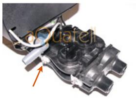
Page 10 Fleck 5600SXT U.S. V1.1 Copyright aQuatell Inc 2010 Metal clips hold the bypass to the turbine. Simply push the bypass onto the turbine assembly and tighten down the metal clips. These clips do not need to be overtightened.
