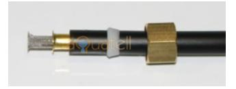
The brass tube insert and woven metal insert must both be pushed fully into the brine line. Once all the pieces have been attached to the brine line push it into the brine line adapter on the valve, and tighten down the brass nut to hold it in place. After completing this make sure that during the process of attaching the brine line to the valve, that the brine tank connection did not loosen.
