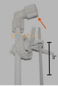
The float assembly controls the flow of brine solution out of the brine tank, and the flow of fresh water into the brine tank. On the thin vertical bar of the float assembly identify the two black rubber washers. These washers control the range of motion of the cup-shaped float.
